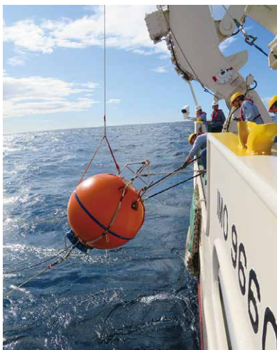
係留流速計の回収作業 Recovery of a mooring of current meter
