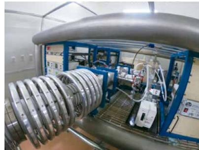
Accelerator Mass Spectrometer, A laser ablation high-resolution inductive plasma mass spectrometer, low background gamma ray spectrometer and other analytical machines.
