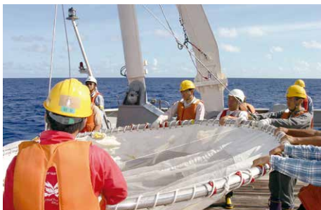
研究船白鳳丸による大型ORIネット作業 Large scaled ORI net operation on board R/V HakuhoMaru to sample fish larvae
