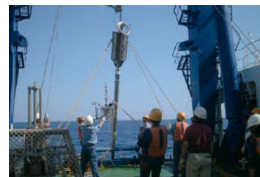
柱状堆積物の採取 Sedimentary core collection
