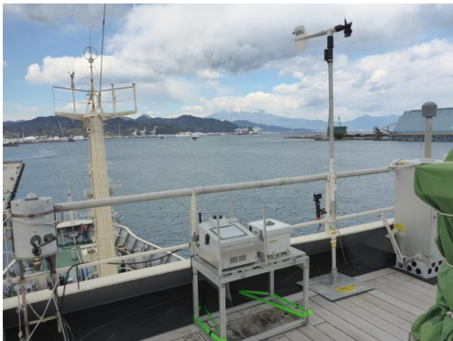
Fig. 1 Microwave radiometer and cloud camera on the deck of Hakuho Maru.
