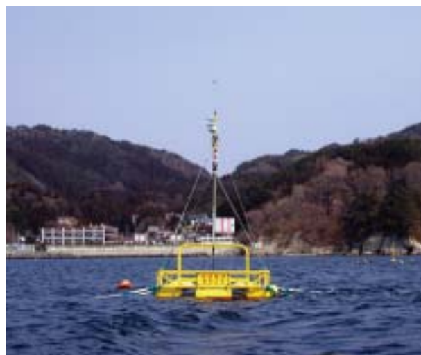
大槌湾に浮かぶ海象観測ブイ。後方に国際沿岸海洋研究センターが見える Telemetering buoy for observing sea water temperature and salinity. International Coastal Research Center can be seen beyond the left side of the buoy
