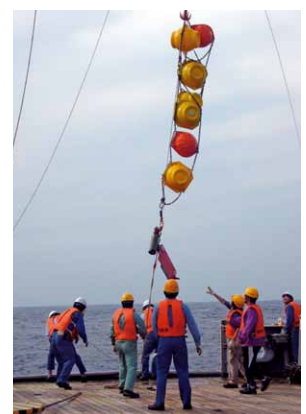
係留流速計の回収作業 Recovery of a mooring of current meter
