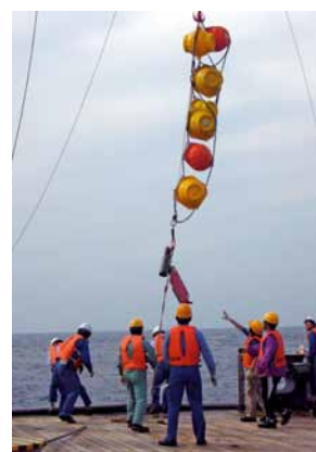
係留流速計の回収作業 Recovery of a mooring of current meter
