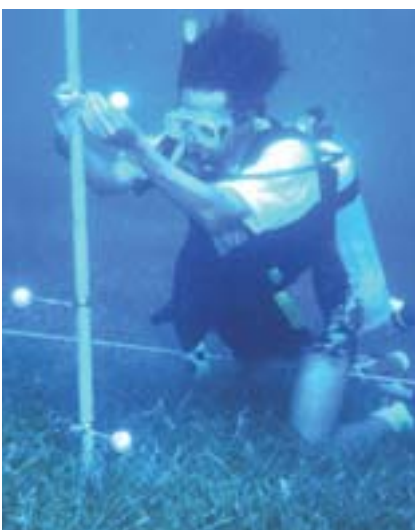
フィジーでの石膏ボールを用いた藻場の流動測定 Diver fixing plaster balls to measure water flow in a seagrass meadow in Fiji
