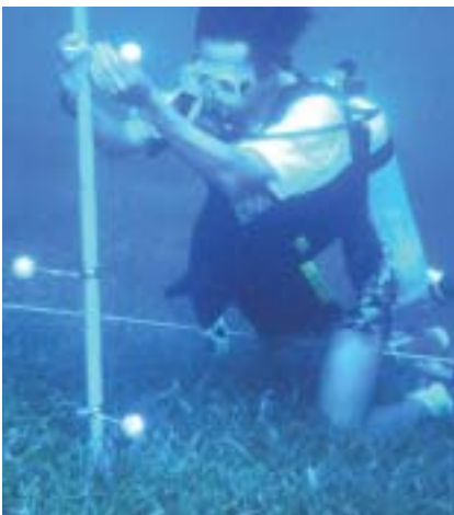
フィジーでの石膏ボールを用いた藻場の流動測定 Diver fixing plaster balls to measure water flow in a seagrass meadow in Fiji
