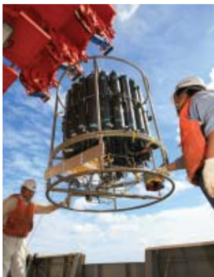
流速と水温、塩分、溶存酸素の測定 Observation of current velocity, water temperature, salinity, and oxygen
