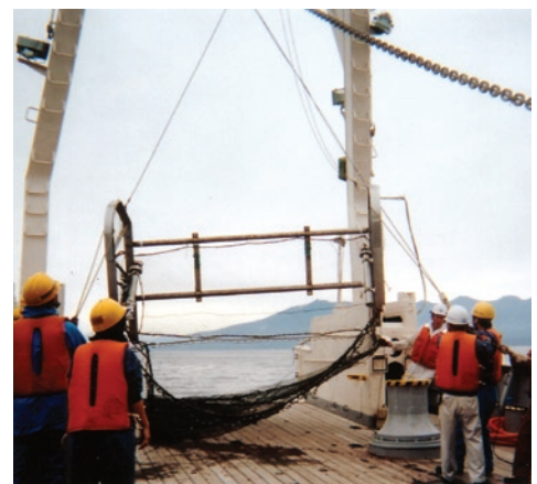
研究船淡青丸でのトロール作業 Sampling of deep-sea benthic animals using a trawl on the R/V Tansai Maru
